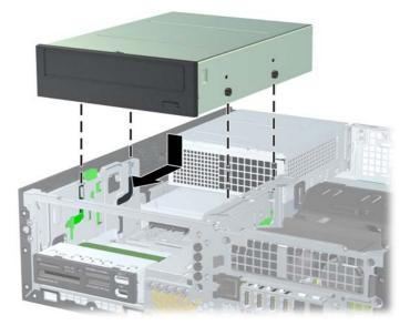
7. Rotate the drive cage to its upright position.
